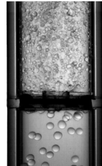
Study of droplet breakup through a calibrated orifice
