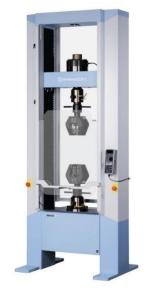
Shimadzu® UTM-600KN according to the ASTM D-882 at a rate of 5 mm/min
