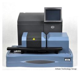
Thermal Analysis SDT Q200 10 °C/min from -30 to 200 °C, with double scanning
