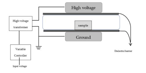
Atmosphere: Air and Nitrogen Conditions: 90 kv during 15 min
