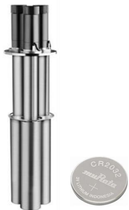
20ml Multicalorimeter (accommodates Coin Cells sizes 2032 and 2325)
