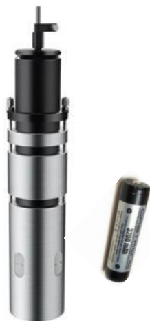
Macrocalorimeter (accommodates 18650 Cells )
